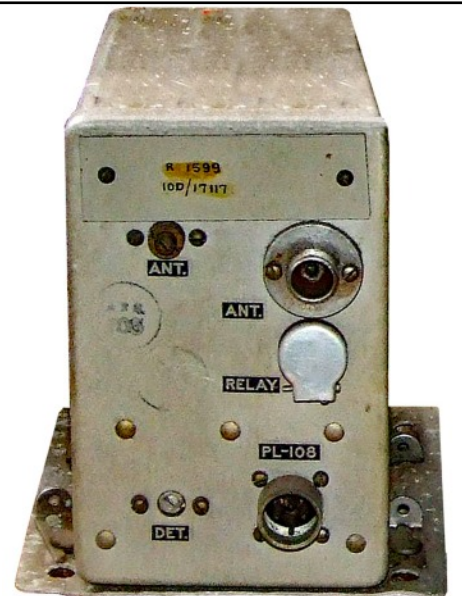
American marker beacon receiver BC-357 (part of RC-43) modified as SBA marker receiver Type R.1599 (above).
